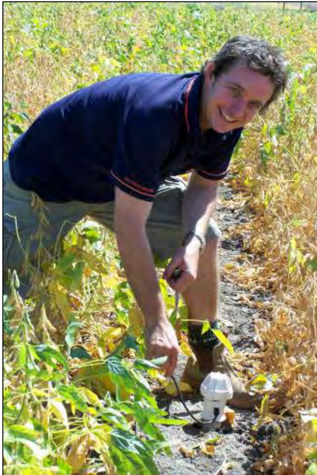
WATER WISE: Luke Gaynor demonstrates the moisture probes in one of David and Paul Bellato's soybean crops which are part of the Better Oilseeds project. Photo: Felicity Pritchard.
